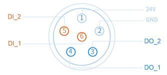
Figure 6.8 Tool I/O interface
